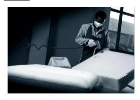
Foaming involves the application of foam materials for comfort and support. The process typically includes the integration of webbing and netting to ensure proper distribution and containment of the foam within the wooden frame. Webbing is used to create a supportive foundation, providing strength and stability to the seating area. Meanwhile, netting acts as a barrier, preventing the foam from shifting or sagging over time
