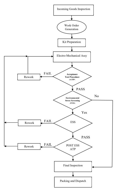
The production process starts once the order is confirmed. The production order will be released by the authorized person against the order and the process type will be defined as either first article inspection ("FAI"). The FAI process will be provided by the customer.
