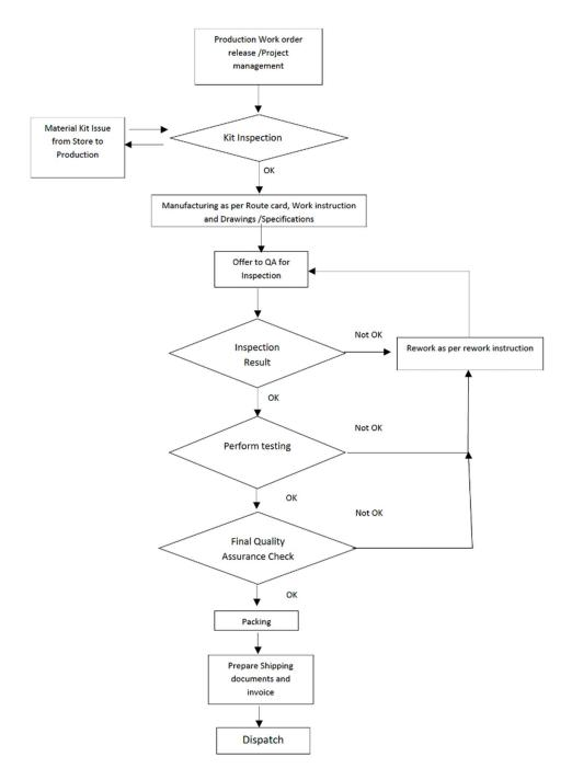
The production process starts once the order is confirmed. The production order will be released by the authorized person against the order and the process type will be defined as either first article or regular production. The FAI process will be performed under the guidance of process engineering team, if required. On-job training will be provided by the customer or internal identified trainer.
