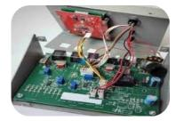
Also known as systems integration, box builds can be anything from a simple PCBA housed in a small enclosure, to a cabinet housing a complex electromechanical system. The box build process involves enclosure fabrication, assembling the various PCBAs and cables harness assemblies, installation of sub-assemblies and components and routing of cabling or wire harnesses.
